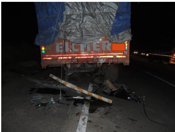
FIGURE 17: Trucks involved in accidents while parked on the shoulders. Inadequate illumination and/or inadequate warnings likely contributed to collisions.
