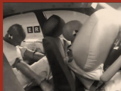
Belted rear occupant held in position in a frontal impact.
