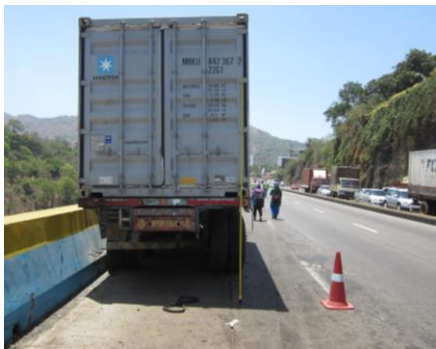
Parked truck on a road section with no shoulder. A truck travelling in the left-most lane collided into it, resulting in fatalities and serious injuries.
